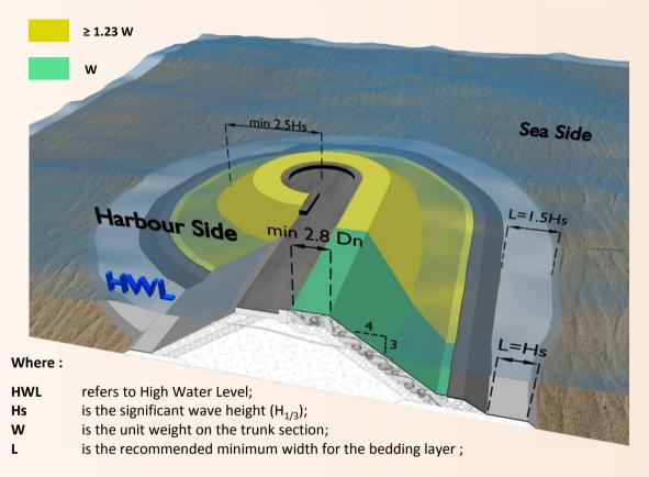
The transition between two sizes of armour unit, in this case the roundhead armour and the trunk armour, is to be built with an angle of 45° in the plane of the underlayer.
