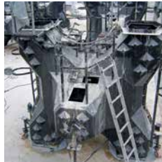
Mould ready for casting
