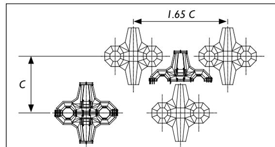
Plan layout of casting arrangement
