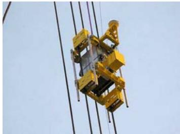
**Figure 4. Cable drum measuring frame**
