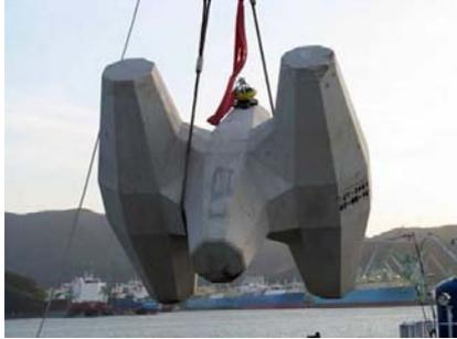
**Figure 3. Measurement box on a CORELOC™ unit**
