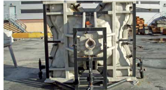
ECOPODE™ shells made of fibre glass embedded in a spider frame
